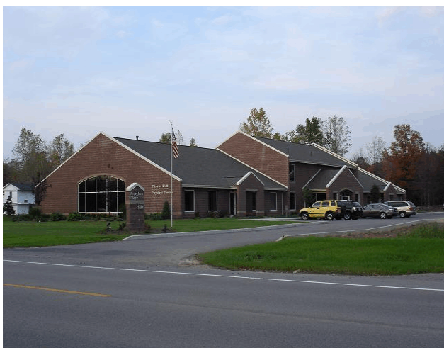
Figure 2.3 Example of preferred parking and circulation system layout. Parking on the side of the building, landscaped area between the street and building, and development signage located at the entrance driveway.
