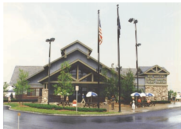
Figure 2.9 Example of design incorporating successful facade base and roof top treatments, and building tenant signage. Design utilizes a variety of roof top treatments and forms to break down the building mass into smaller human scale elements.
